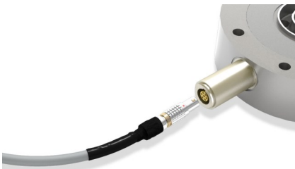
► Plug-in cable connection with shielded measuring cable type SMC (S-CAB-L-5M-F), always with straight connector plug.
